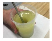
5. Mix with wing stirrer thoroughly for 1 minute until material is homogeneous
