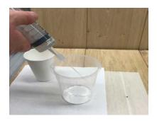
3. Put 25 ml of water (enough for 300 ml WAKOL MS 335 Repair Resin) with the syringe into the measuring cup
